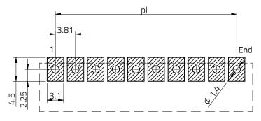
Stencil thickness: 120 µm
