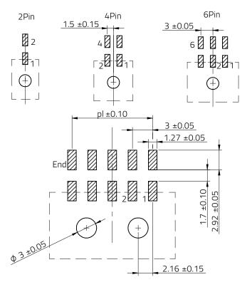
Max Recommended PCB Thickness: 1.6mm
