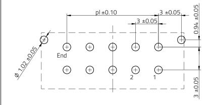
Max. Recommended PCB Thickness: 1.6mm
