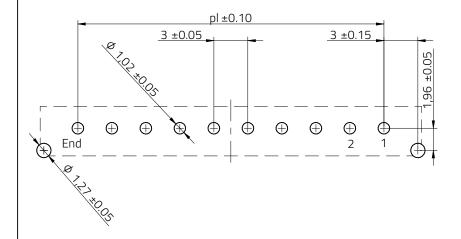
Max. Recommended PCB Thickness: 1.6mm
