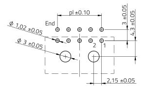
Max. Recommended PCB Thickness: 1.6mm
