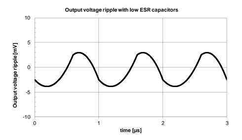
When capacitors with slightly higher ESR are utilized, the dominant parameter which influences the output voltage ripple is just the ESR:
