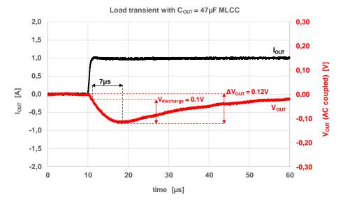
The  $\Delta V_{OUT} = 0.12V$  and  $t_d = 7\mu s$ . It is important to remind that the  $\Delta V_{OUT}$  includes also the voltage drop during  $t_{rise}$ , mainly due to the ESR (V<sub>ESR</sub> = 20mV, see picture above). In order to achieve the desired maximum  $\Delta V_{OUT}$ , the V<sub>discharge</sub> should be below 0.06V. Using the equation (9), the minimum required output capacitor is:
