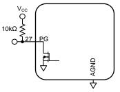
$V_{CC} = V_{IN}$  or other supply voltage below 6V
