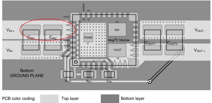
The negative terminal of  $C_{IN1}$  and  $C_{IN2}$  need to be very close to the PGND pad of the power module. The ground path is passing through the vias at the  $C_{IN}$  terminals and thermal vias around the PGND pad.
