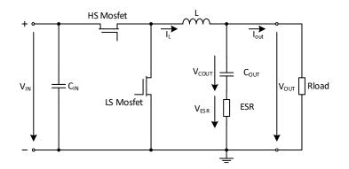
None of the required output capacitors are integrated within the module. The output capacitor must meet the worst case RMS current rating of  $0.5 * \Delta I_L$ , as calculated in equation (4).
