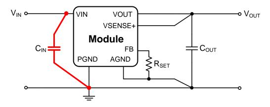
Based on those considerations, the path of the input capacitor  $C_{IN}$  is the most critical one to generate high frequency noise on  $V_{IN}$ . Therefore place  $C_{IN}$  as close as possible to the Magl<sup>3</sup>C power module  $V_{IN}$  and PGND pins. This will minimize the high di/dt area and reduce radiated EMI. Additionally, grounding for both the input and output capacitor should consist of a localized top side plane that connects to the PGND pins.
