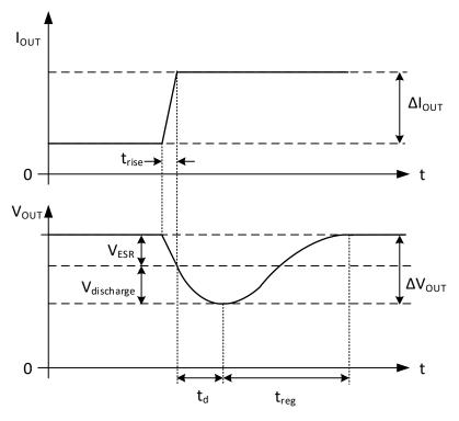
The second contributing factor is the voltage drop due to discharge of the output capacitor, which can be estimated as:
