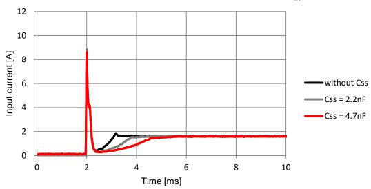
Input current at start up with different soft-start capacitors -  $V_{IN} = 5V$
