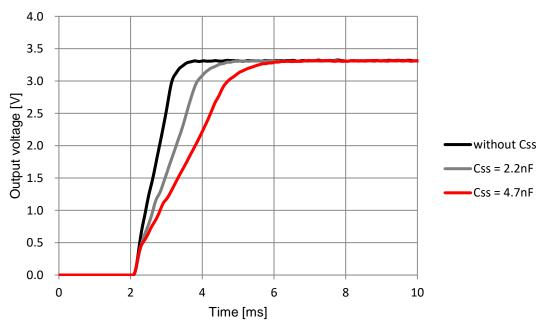
Output voltage at start up with different soft-start capacitors -  $V_{IN} = 5V$
