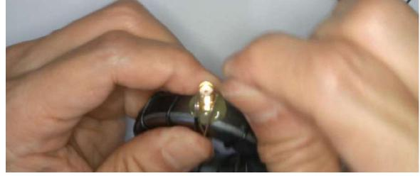
Solder the copper wire to SMA connector carefully. Do not put too much solder on the SMA connector to avoid covering the screw thread.
