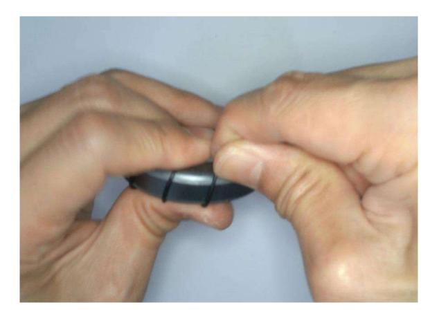
Wind the wire between 8 to 12 turns around the ferrite
