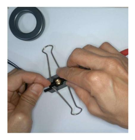
Press on the J-hook to secure it to SMA connector pin
