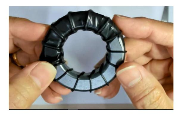
Wrap one round of PVC tape to the Part 1 ferrite core
