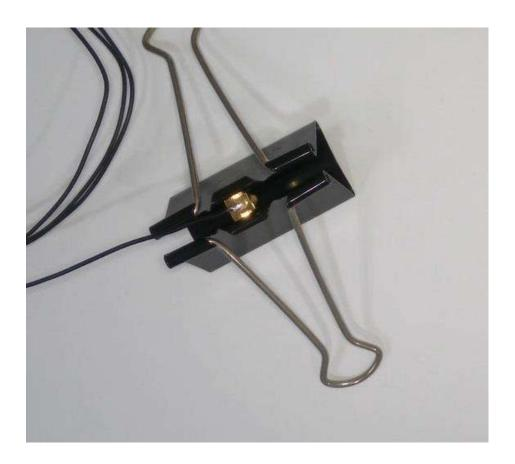
Inspect SMA connector pin solder quality
