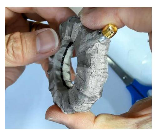
Paste the 4cm X 2.5cm fabric shielding around the inner core in such a way that it leaves a small even gap of (1~2mm) in the middle of the ferrite inner core
