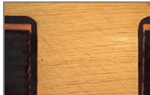
Cut view of press-fit area
