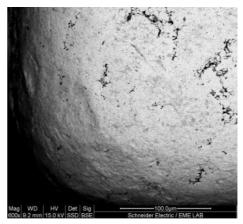
Figure 7: SEM image of tin surface after 1500 h, RH 93 %, 55  $^{\circ}\mathrm{C}$
