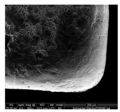
Figure 6: SEM image of tin surface before test
