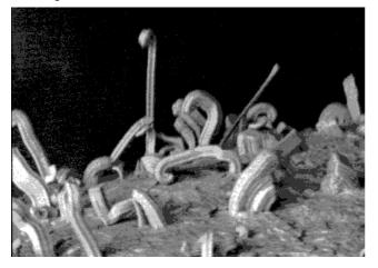
Figure 1: Whisker formation on Tin surface (reprinted with permission of NASA Electronic Parts & Packaging (NEPP) Program
