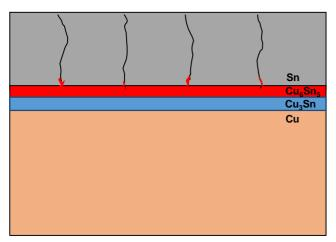
Figure 5: Formation of Cu<sub>3</sub>Sn by annealing
