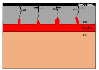
Figure 4: Stress induced by oxygen growth
