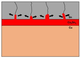
Figure 3: Stress induced by grain boundary diffusion
