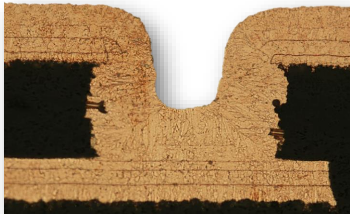
No defects after 1000 cycles
