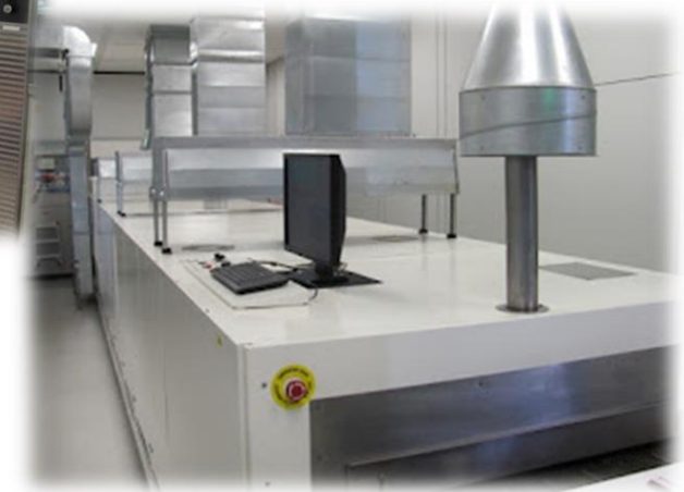
Curing of the polymer
