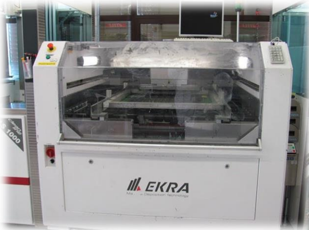
Alignment of the polymer printing to the etched layout (with Fiducials on the edges of the productions panel)
