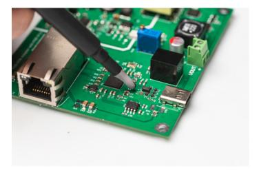
Noise source detection with **Near Field probes.**
