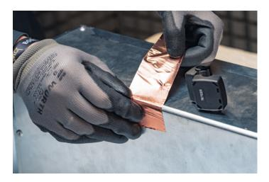
Shielding optimization of an enclosure using adhesive **Copper tape.**
