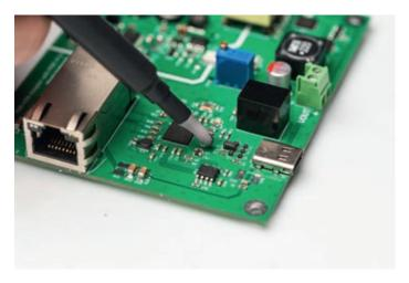
Noise source detection with **Near Field probes.**
