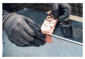
Shielding optimization of an enclosure using adhesive **Copper tape.**
