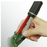
PCB circuit conductivity test
