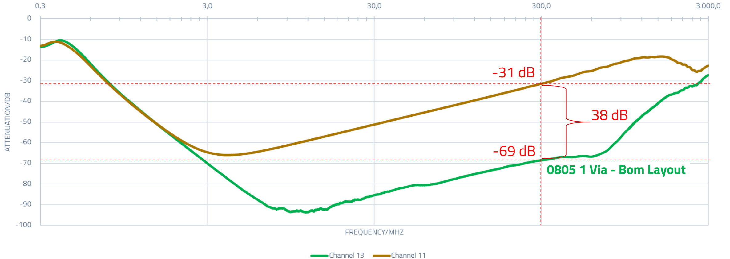
S21 Insertion Loss (R&S ZNB20 VNA)
