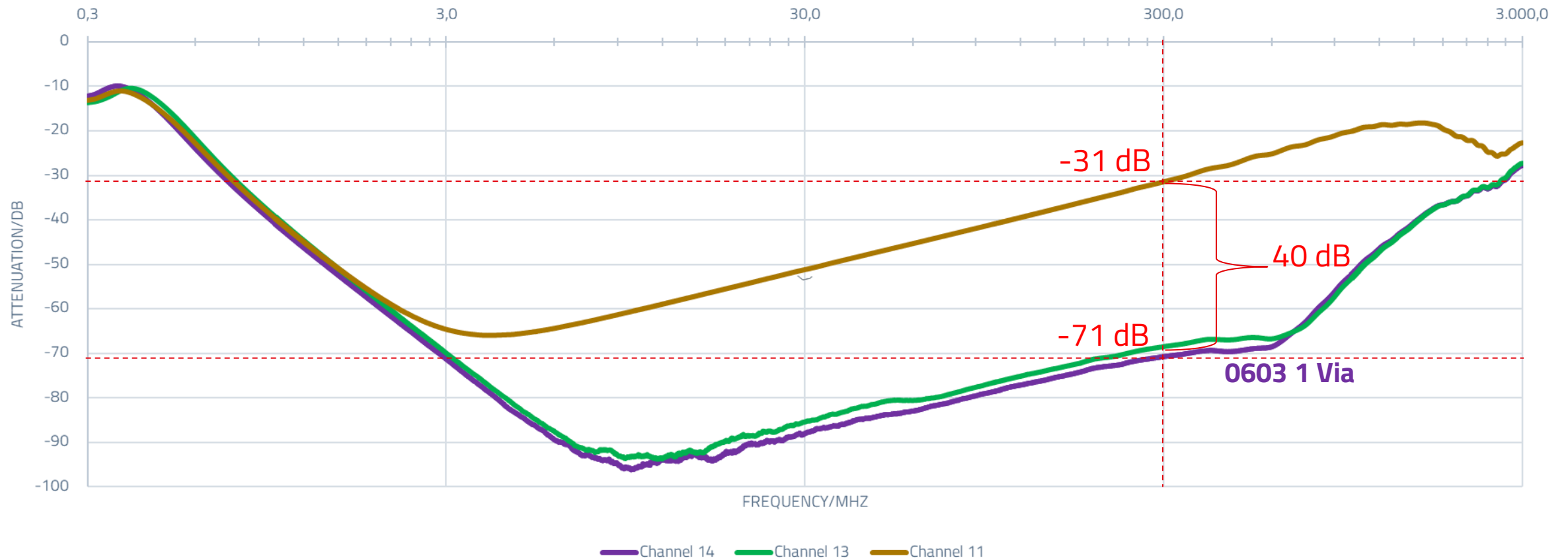
S21 Insertion Loss (R&S ZNB20 VNA)
