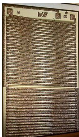
Figure 5: Dual output transformer for GaN gate drive.
