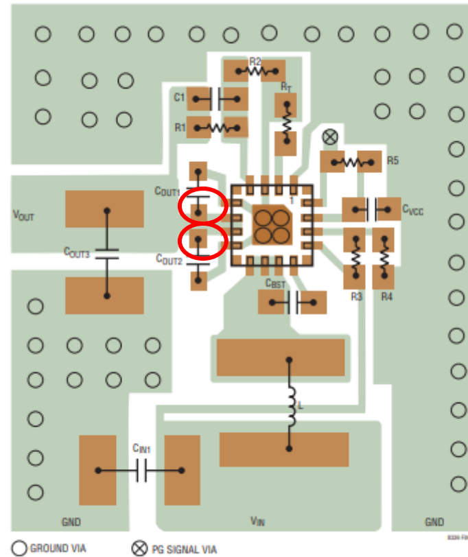
Figure 4. A Recommended PCB Layout for the LT8336
