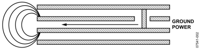
Figure 2. Edge Radiation From an Edge Matched Ground Power Pair
