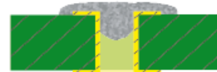
Solder paste fills the stencil's aperture
