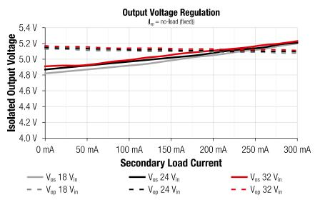
Figure 17: Voltage Regulation (at fixed  $I_{os}$  = no-load (unbalanced load))
