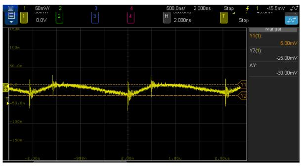
Figure 28: Primary output voltage ripple (@  $V_{in} = 24$  V,  $I_{op} = I_{os} = 300$  mA (balanced full-load))
