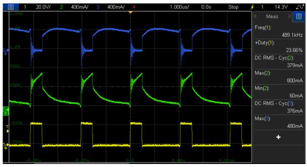
Figure 26: Winding currents and SW node voltage (@  $V_{in} = 24 V$ ,  $I_{op} = I_{os} = 300 mA$  (balanced full-load)) ( $I_{os}$ ,  $I_{op}$ ,  $V_{SW}$ )
