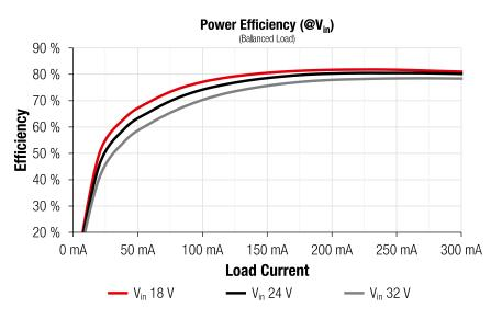
Figure 19: Power Efficiency (balanced load)
