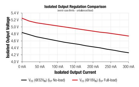
Figure 18: Voltage Regulation worst-case limits (unbalanced load)
