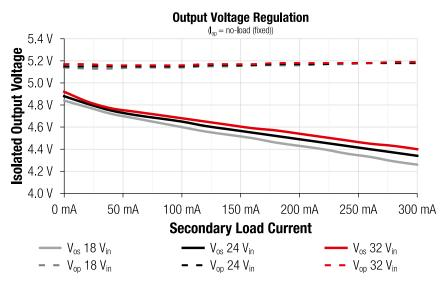
Figure 15: Voltage Regulation (at fixed  $I_{op}$  = no-load (unbalanced load))
