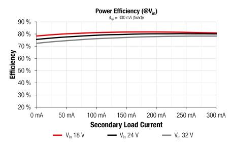
Figure 20: Power Efficiency (at fixed  $I_{op} = 300$  mA (unbalanced load))
