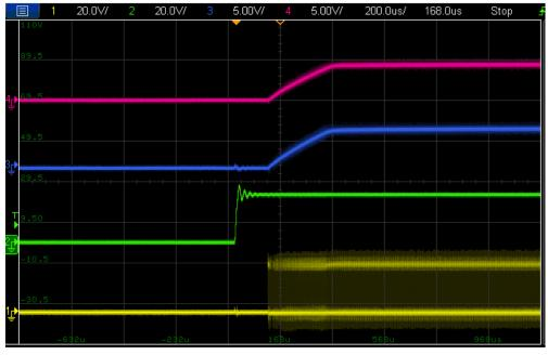
Figure 24: Start-up characteristic ( $V_{in} = 24 V$ ,  $I_{op} = I_{os} = 300 mA$  (full-load, balanced)) ) ( $V_{os}$ ,  $V_{op}$ ,  $V_{in}$ ,  $V_{sw}$ )
