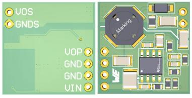
Figure 9: RD006 Board 3D detail: top side (left)(top view), bottom side (right)(bottom view)
