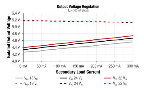
Figure 16: Voltage Regulation (at fixed  $I_{0s} = 300$  mA (unbalanced load))
