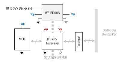
Figure 7: Isolated RS-485 transceiver system (simplified)
