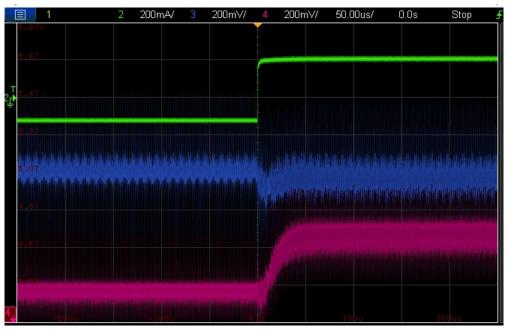
Figure 34: Load transient – Rising step (I<sub>os</sub> = 300 mA, Primary load current step from 0 mA to 300 mA, 1 A/µs) (V<sub>os</sub>, V<sub>op</sub>, V<sub>in</sub>)
