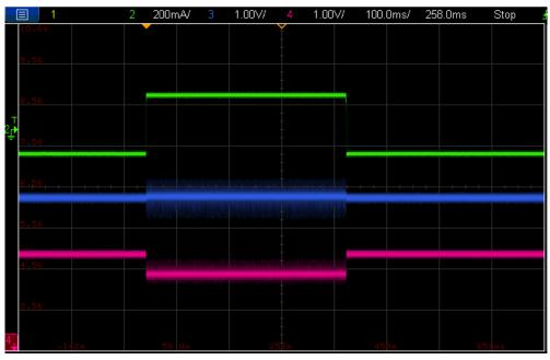
Figure 32: Load transient ( $I_{op}$  = no-load, Secondary load current step 0 to 300 mA, 1 A/µs) ( $V_{os}$ ,  $V_{op}$ ,  $V_{in}$ )
