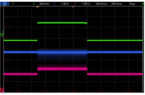
Figure 30: Load transient ( $I_{os}$  = no-load, Primary load current step 0 to 300 mA, 1 A/µs) ( $V_{os}$ ,  $V_{op}$ ,  $V_{in}$ )
