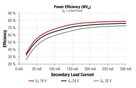
Figure 23: Power Efficiency (at fixed I<sub>os</sub> = no-load (unbalanced load))
