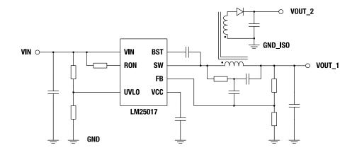
Figure 2: Simplified schematic
