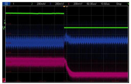
Figure 35: Load transient - Falling step (I<sub>os</sub> = 300 mA, Primary load current step from 300 mA to 0 mA, 1 A/µs) (V<sub>os</sub>, V<sub>op</sub>, V<sub>in</sub>)
