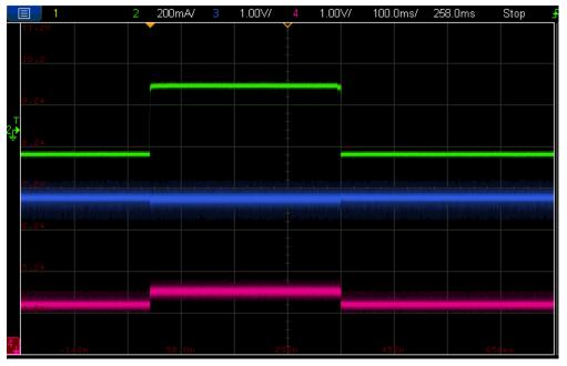
Figure 31: Load transient ( $I_{os}$  = 300 mA, Primary load current step 0 to 300 mA, 1 A/µs) ( $V_{os}$ ,  $V_{op}$ ,  $V_{In}$ )
