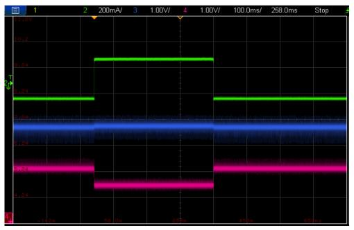
Figure 33: Load transient (Iop = 300 mA, Secondary load current step 0 to 300 mA, 1 A/µs) (Vos, Vop, Vin)
