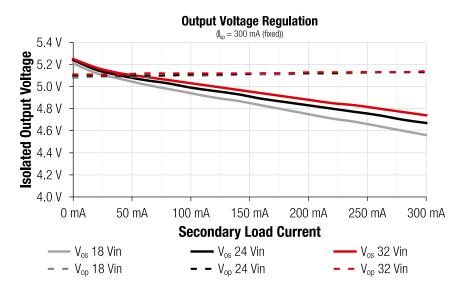
Figure 14: Voltage Regulation (at fixed  $I_{op} = 0.3$  A (unbalanced load))
