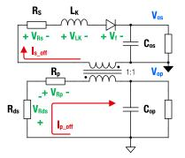
Figure 4: Equivalent circuit with parasitic elements during OFF-time of Q1 (open)
