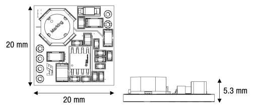
Figure 11: RD006 Board Dimensions: board sides (left), board height (with 1.5 mm thick PCB) (right)
