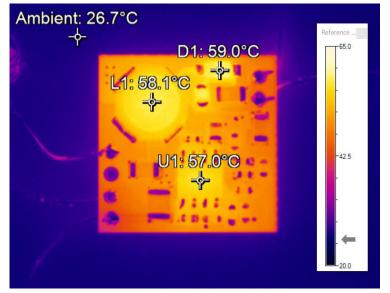
Figure 37: Board components temperature at  $V_{in}$  (nom) = 24 V and 25 °C ambient
