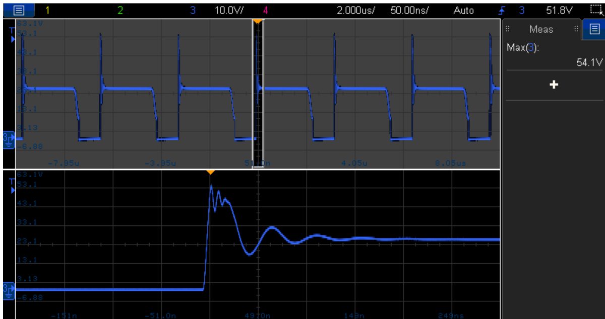
Figure 21: SW Node voltage clamping ( V_{in} = 18\text{ V} , P = 6\text{ W} )
