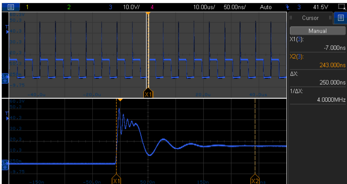
Figure 22: SW Node ringing damping ( V_{in} = 9\text{ V} , P = 6\text{ W} )
