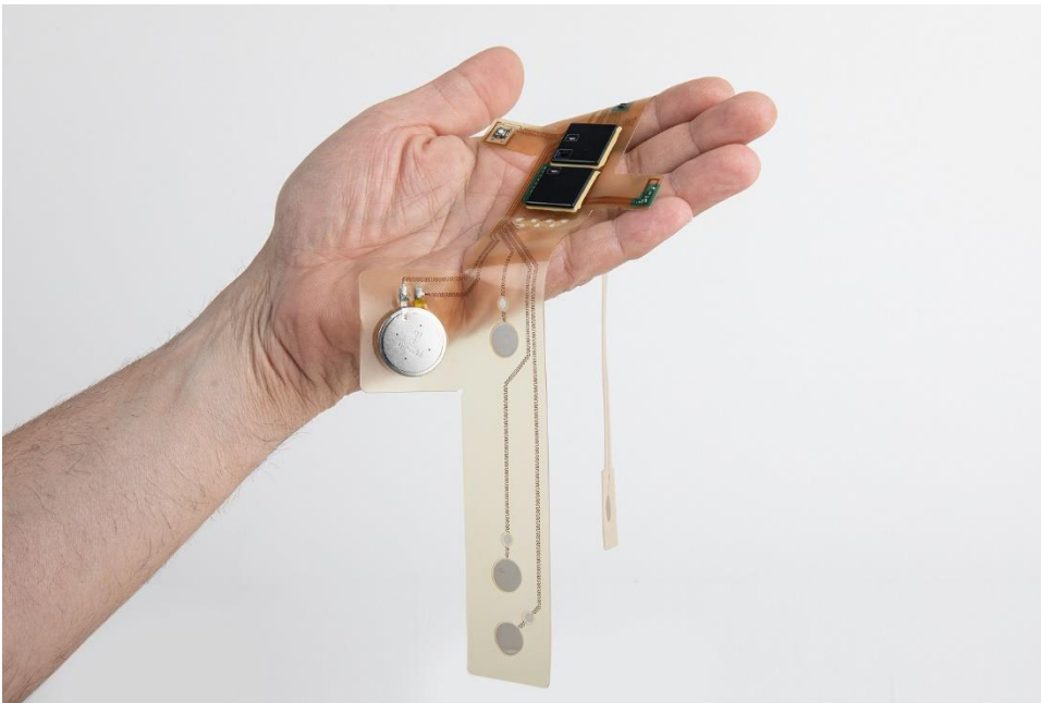
Picture 1: Stretchable printed circuit board with integrated electronics and printed electrodes – a very pliable, biocompatible substrate for smart patches. (Source: Würth Elektronik Circuit Board Technology)
