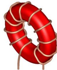
$$\begin{aligned}\underline{Z}(f) &= \underline{Z}_0(f) \cdot \underline{\mu}_r(f) \\ &= j \cdot 2\pi \cdot f \cdot L_0 \cdot [\mu'_r(f) - j \cdot \mu''_r(f)] \\ &= j \cdot X_L(f) + R(f)\end{aligned}$$
