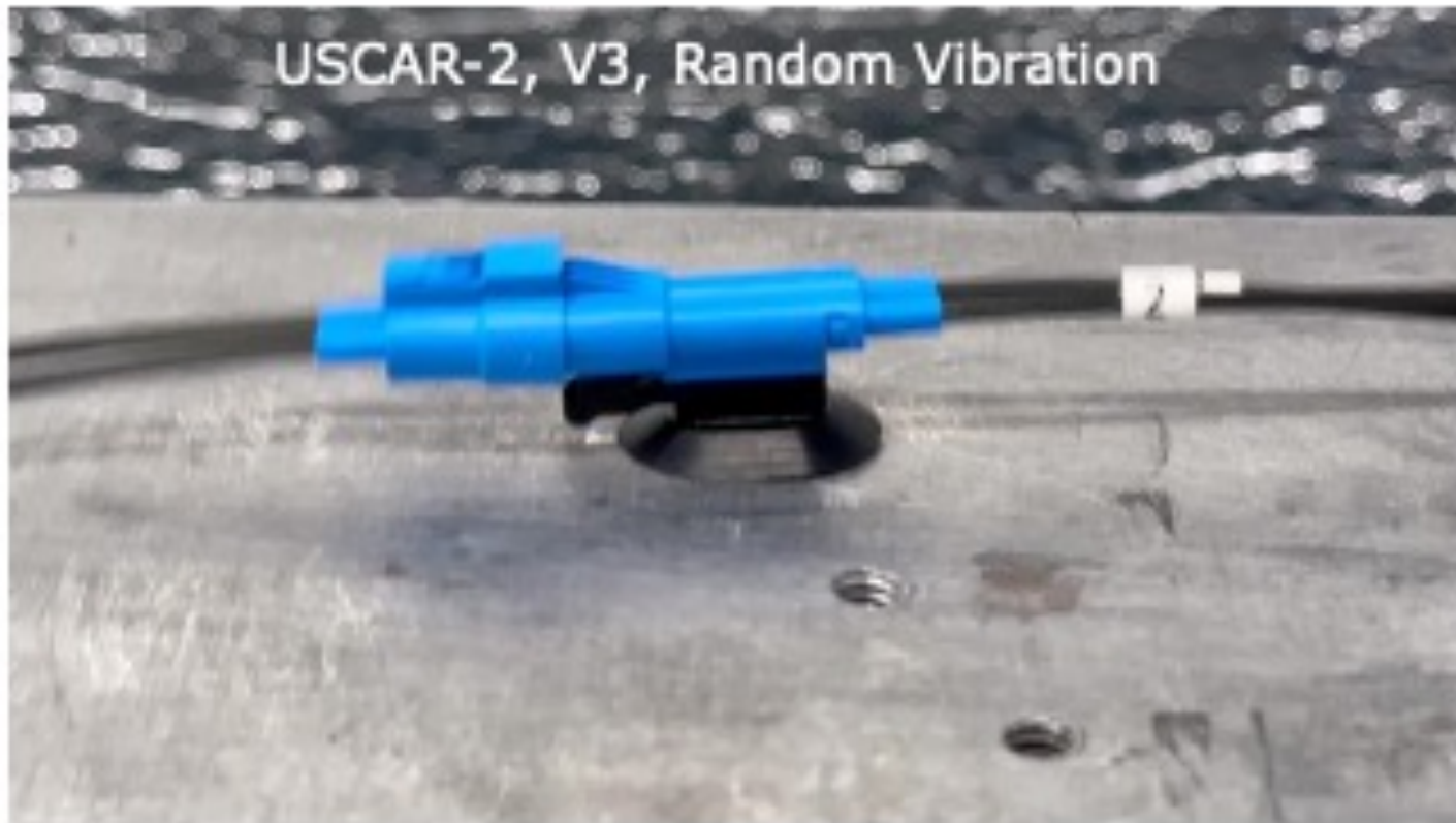
Connector in vibration (random) testing
