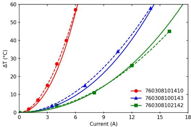
**Fig. 3** Comparison of the interpolated measured rated current curves (dashed lines) and calculated rated current curve (solid lines) with  $\alpha=12 \text{ W}/(\text{m}^2\text{K})$ .
