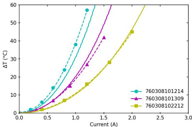
**Fig. 4** Comparison of the interpolated measured rated current curves (dashed lines) and calculated rated current curve (solid lines) with  $\alpha=21.3 \text{ W}/(\text{m}^2\text{K})$ .
