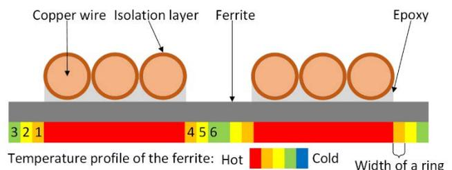
**Fig. 1** Cross section of the used physical model of a WPT coil with the temperature distribution of the ferrite rings.
