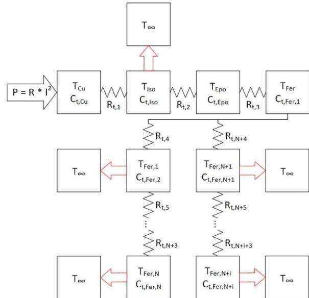
**Fig. 2** Equivalent electrical circuit of the physical WPT coil model. The blocks  $T_{Fer,1}$  to  $T_{Fer,N+i}$  represent ferrite rings. The red arrows indicate the heat dissipation caused by thermal radiation and convection.  $T_\infty$  is the ambient temperature.
