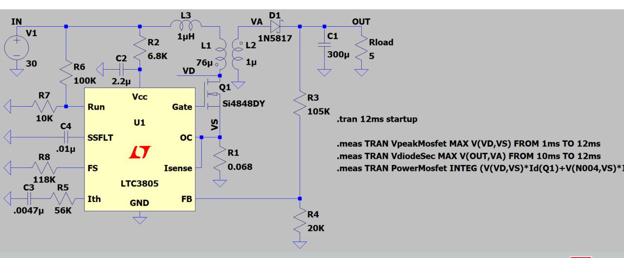
.meas TRAN VpeakMosfet MAX V(VD,VS) FROM 1ms TO 12ms
