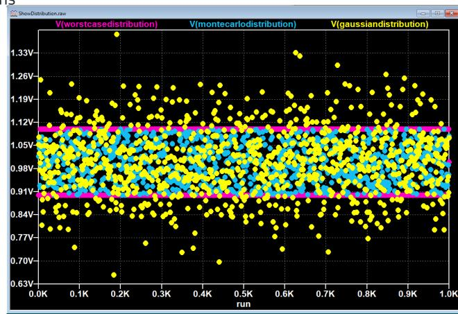
.func wc(nom,tol,index) if(run==numruns,nom,if(binary(run,index),nom\*(1+tol),nom\*(1-tol))) .func binary(run,index) floor(run/(2\*\*index))-2\*floor(run/(2\*\*(index+1)))
