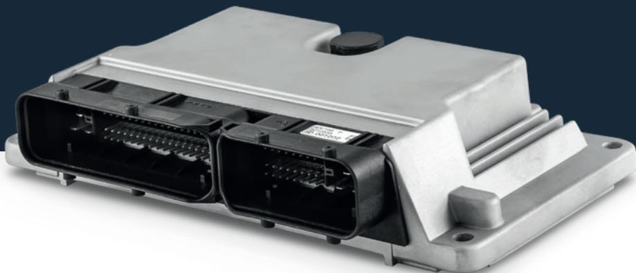
The **ICCS CAN Controller 121P** is part of the Intelligent Control and Command Systems (ICCS) product range. It can be easily integrated into your CAN network or used as a standalone module. The 16-bit NXP HCS12XEQ processor with integrated co-processor has sufficient computing power to handle complex tasks. The two CAN and an optional LIN master interface allow data exchange between independent bus systems or enable gateway / filter functions.
