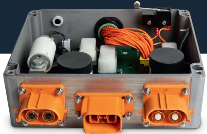
The high voltage power distribution unit (HV PDU) is a central element of the electrical architecture in an electric vehicle. It establishes the electrical connection between the battery, on-board charger, motor and other consumers such as heaters, DC-DC converters, etc.
