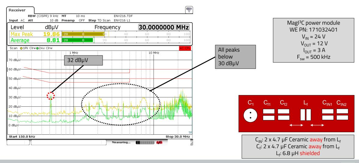
Placement of input filter components; possible options
