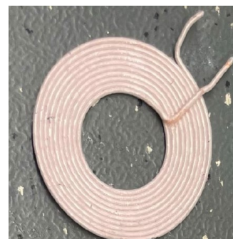
Fig. 3 Winded coil in accordance to the Qi-A11 design [4]
