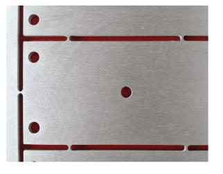
**Positive micro edges** The breaking point is located in the rout path outside the PCB outline.
