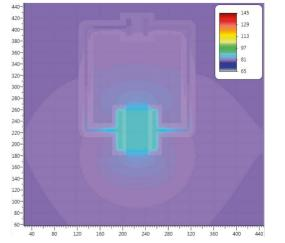
Printed circuit board 2 layer, 1,6 mm, improved layout, without thermal vias
