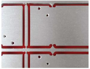
**Negative micro edges** Breaking point inside the PCB outline. To ensure stability of the panel additional ribs are required.
