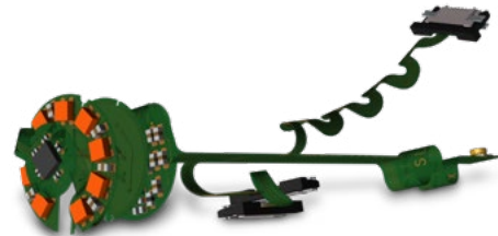
SLIM.flex 4F-Ri in Anylayer microvia technology
