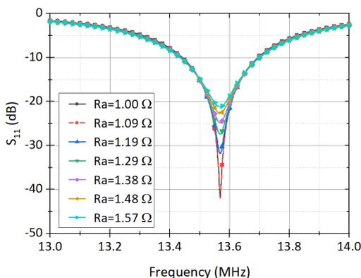
**Fig. 9:**  $S_{11}$  magnitude in dependence on the frequency for different NFC antenna resistances.
