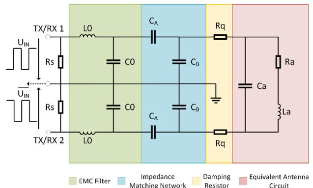
**Fig. 3:** Differential output NFC circuit. [7]
