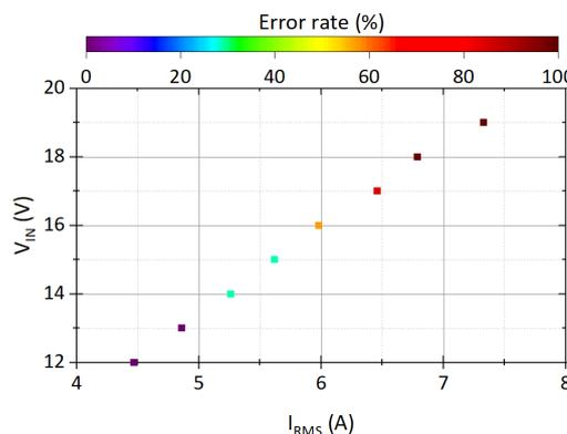
**Fig. 8:** NFC error rates for different RMS currents in the Tx WPT coil.
