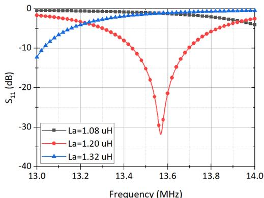
**Fig. 12:** Reflection coefficient magnitude vs. frequency within the NFC antenna inductance tolerance.
