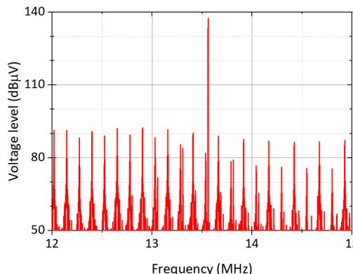
**Fig. 7:** FFT of the Rx NFC antenna during standby and an active WPT system.
