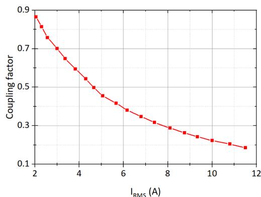
**Fig. 5:** Measured coupling between the WPT coils at the Tx and Rx side in dependence of the Tx RMS current with  $V_{\text{in}} = 12 \text{ V}$ .
