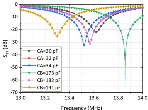
**Fig. 11:**  $S_{11}$  magnitude vs. frequency for impedance matching circuit components tolerances.
