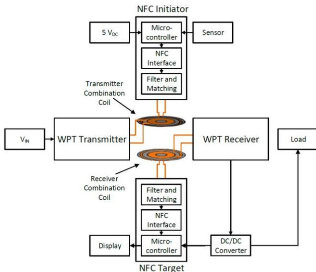
**Fig. 2:** Block diagram of the developed simultaneous WPT/NFC system.
