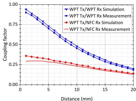
**Fig. 4:** Simulated and measured coupling factor of the WPT Tx coil, the Rx coil and the NFC target antenna for different distances for the product 760308101150.
