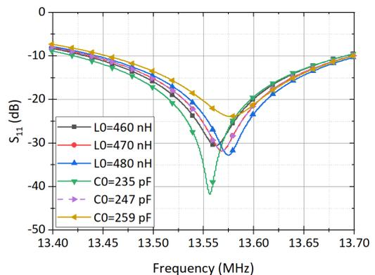
**Fig. 10:** Reflection coefficient vs. frequency for EMC filter components tolerances.
