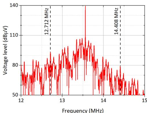
**Fig. 6:** FFT of the Rx NFC antenna during data transmission without an active WPT system.
