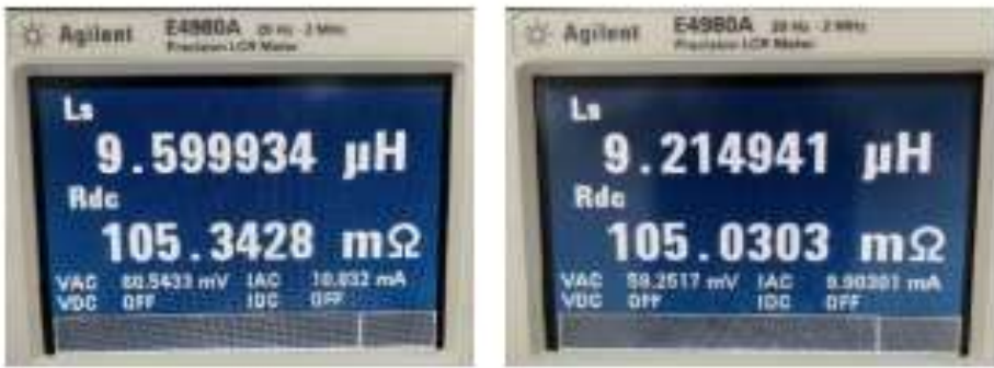
Figure 6: RDC and inductance measurement of component without voltage defect (left) and with voltage defect (right)
