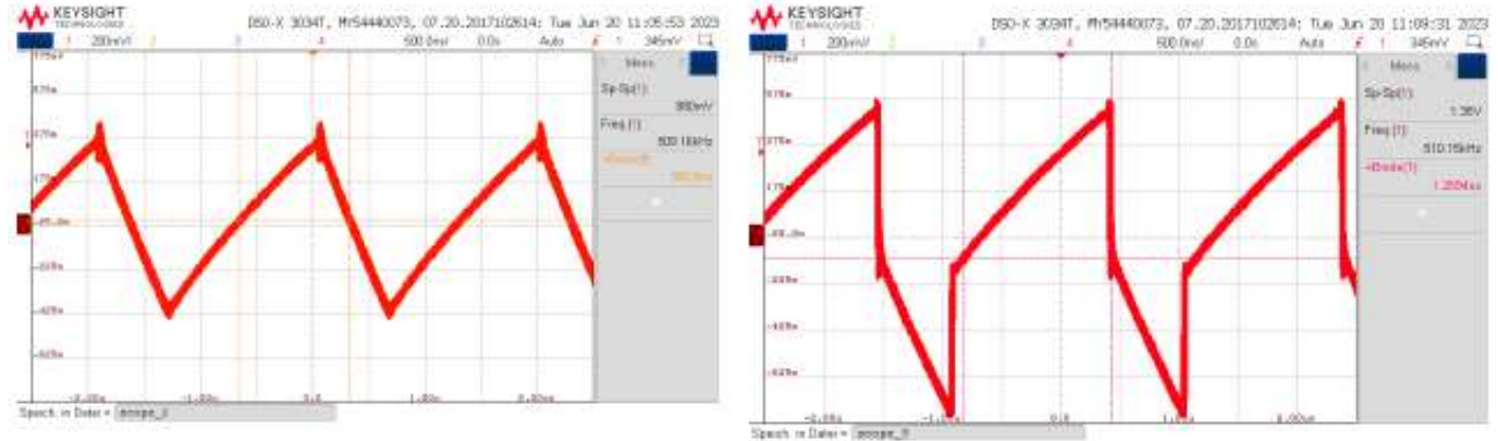
Figure 8: Screen capture of the ripple current undamaged component (left) and damaged component (right)
