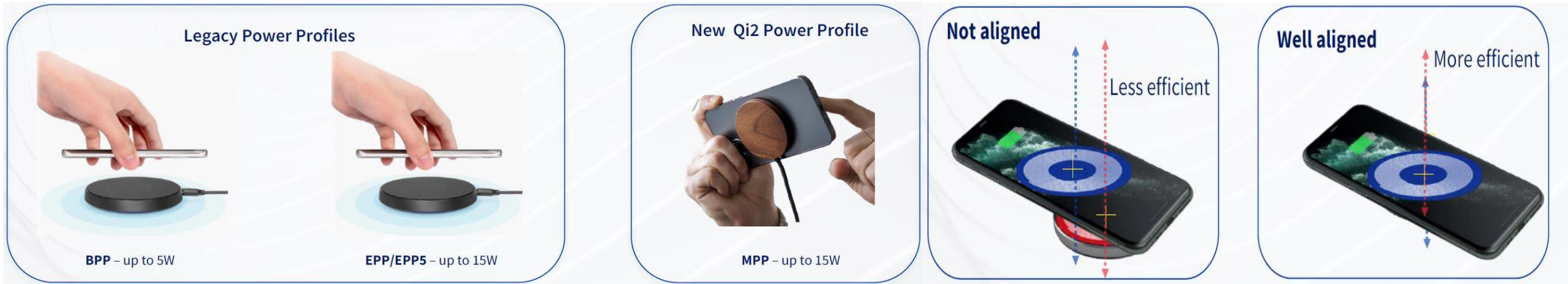
Figure 11: Advantage of using Qi2 Power Profile over the Legacy Qi Power Profile
