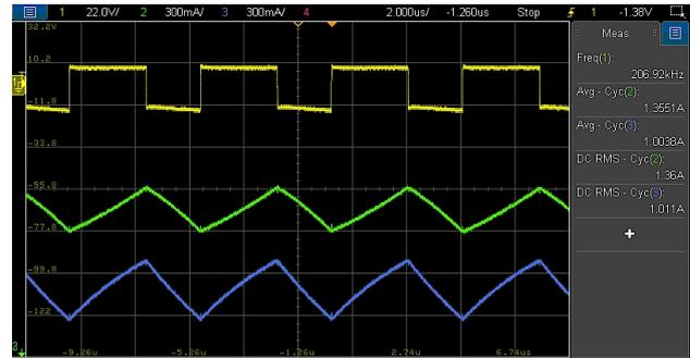
Figure 60: CCM-SEPIC measurements with WE-MCRI ( $L_k=24$   $\mu$ H) and  $C_{AC} = 1.5$   $\mu$ F at  $I_{out}=1$  A ( $V_{L1}$  (I),  $L1$  (II),  $L2$  (II))
