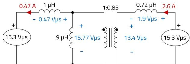
Figure 50: Calculated volt-seconds and ripple currents ( $k=0.9$ ,  $n=0.85$ )
