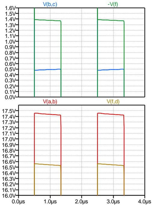
Figure 46: Simulation results: voltages across  $L_{1k}$  (blue),  $L_{2k}$  (green),  $L_{1m}$  (red),  $L_{2m}$  (brown), during  $\Delta t_{on}=0.85 \mu s$  showing two switching cycles (LTspice™) ( $k=0.9, n=0.95$ )
