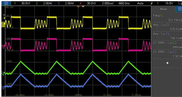
Figure 24: Measured  $L_1$ ,  $L_2$  waveforms of DCM-SEPIC ( $I_{L1}$  ()),  $V_{L1}$  (I),  $I_{L2}$  ()),  $V_{L2}$  (I))
