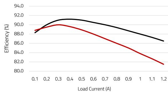
Figure 61: CCM-SEPIC Efficiency results with  $C_{AC} = 1.5$   $\mu$ F and WE-MCRI 47  $\mu$ H with  $k=0.995$  (red) and  $k=0.7$  (black)
