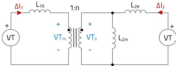
Figure 47: Coupled inductor T-model circuit (alternative version)
