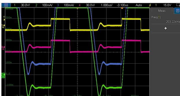
Figure 25: Measured  $L_1$ ,  $L_2$  waveforms of DCM-SEPIC with damped oscillation and zoomed  $I_{LD}$  detail ( $I_{L1}$  ()),  $V_{L1}$  (I),  $I_{L2}$  (I),  $V_{L2}$  (I))
