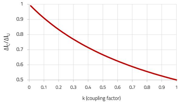
Figure 38: SEPIC: Ripple current ratio vs coupling factor
