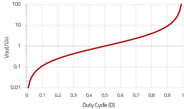
Figure 7: Ideal voltage conversion ratio of SEPIC
