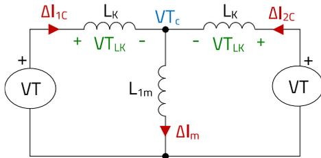
Figure 37: Coupled inductor equivalent circuit (identical windings)
