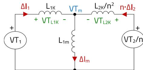
Figure 36: Coupled inductor equivalent circuit
