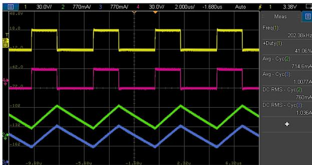
Figure 33: CCM-SEPIC measurements with two separate 47  $\mu\text{H}$  inductors (WE-PD-744770147) at  $I_{out}=1\text{A}$  ( $I_{L1}$  (I),  $V_{L1}$  (V),  $I_{L2}$  (I),  $V_{L2}$  (V))
