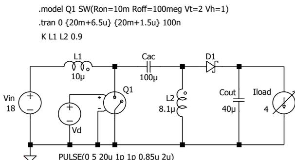
Figure 48: LTSpice™ setup with K directive ( $k=0.9$ ,  $n=0.9$ )
