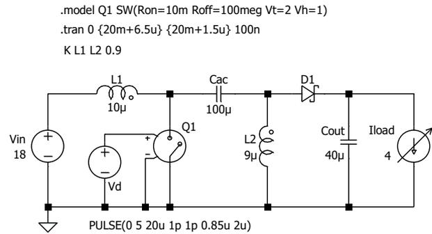
Figure 42: LTSpice™ setup with 'K' directive ( $k=0.9$ ,  $n=0.95$ )
