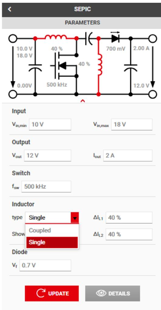
Figure 62: REDEXPERT™ module for SEPIC magnetics selection
