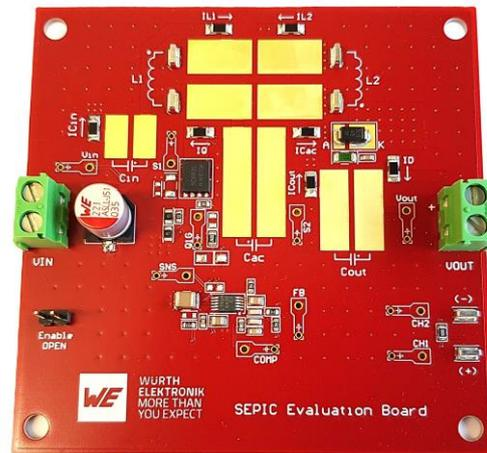
Figure 66: DC-DC SEPIC Prototype board used for measurements
