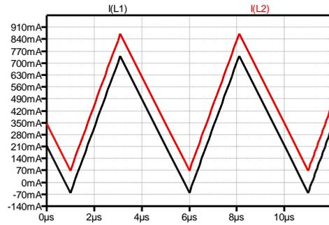
Figure 17:  $L_1, L_2$  currents for  $I_{out} = 0.47\text{ A}$  (CCM-Boundary) (LTspice™)
