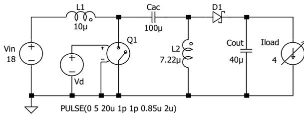
Figure 51: LTSpice™ setup with  $K$  directive ( $k=0.9$ ,  $n=0.85$ )
