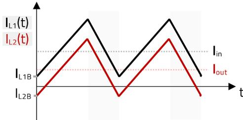
Figure 16: Boundary CCM-DCM of SEPIC for  $V_{out} > V_{in}$
