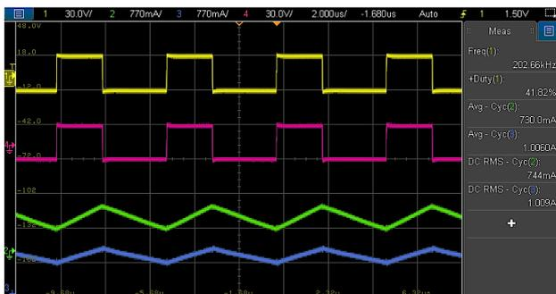
Figure 34: CCM-SEPIC measurements with a 47  $\mu\text{H}$  coupled inductor (MCRI-7448991470) with  $k=0.995$  at  $I_{out}=1\text{A}$  ( $I_{L1}$  (I),  $V_{L1}$  (V),  $I_{L2}$  (I),  $V_{L2}$  (V))
