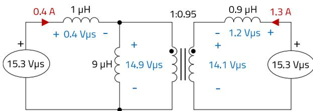
Figure 44: Calculated volt-seconds and ripple currents ( $k=0.9, n=0.95$ )
