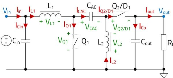
Figure 6: SEPIC reference schematic for current/voltage polarities
