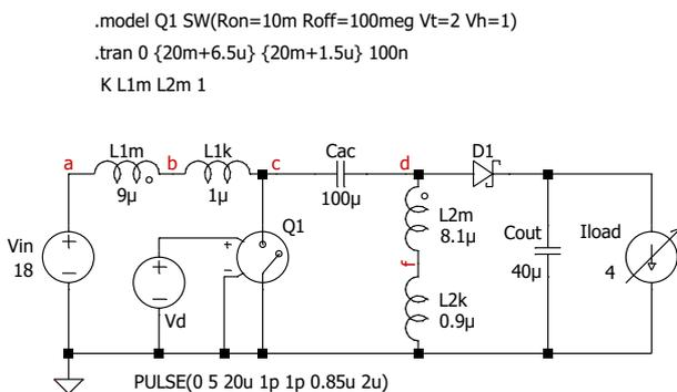
Figure 41: LTSpice™ setup with discrete inductances ( $k=0.9$ ,  $n=0.95$ )
