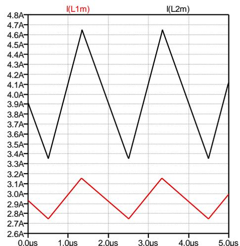
Figure 43: LTSpice™ simulation results ( $I_{L1}$  (red),  $I_{L2}$  (black))
