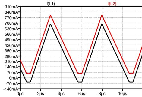
Figure 18:  $L_1, L_2$  currents for  $I_{out} = 0.4\text{ A}$  (DCM) (LTspice™)
