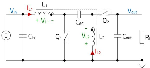
Figure 31: Schematic of SEPIC with magnetically coupled windings
