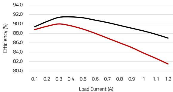
Figure 58: CCM-SEPIC Efficiency results with WE-MCRI-7448991470 ( $L_k=370$  nH) with  $C_{AC} = 1.5$   $\mu$ F (red) and  $C_{AC} = 15$   $\mu$ F (black)
