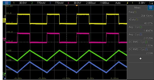
Figure 10: Measured  $L_1$ ,  $L_2$  CCM waveforms ( $I_{L1}$  (I),  $V_{L1}$  (V),  $I_{L2}$  (I),  $V_{L2}$  (V))
