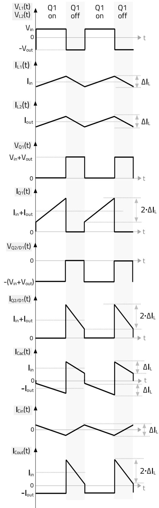
Figure 9: Main circuit waveforms of CCM SEPIC
