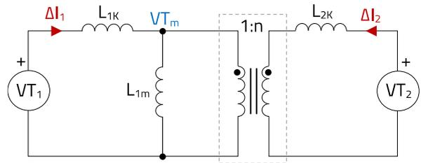
Figure 35: Voltage driven coupled inductor windings: 'T-model' circuit
