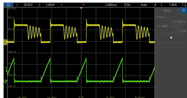
Figure 26: Measured  $Q_1$  waveforms of DCM-SEPIC ( $V_{Q1}$  ()),  $I_{Q1}$  (I))
