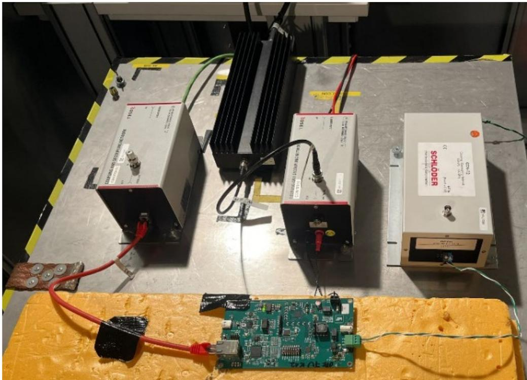
Figure 19: Conducted immunity testing of the PSE board.
