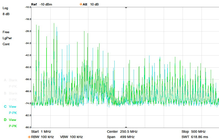
Figure 8: Shielding attenuation, blue: well-known manufacturer available in electrical markets, green: Asian online trade.
