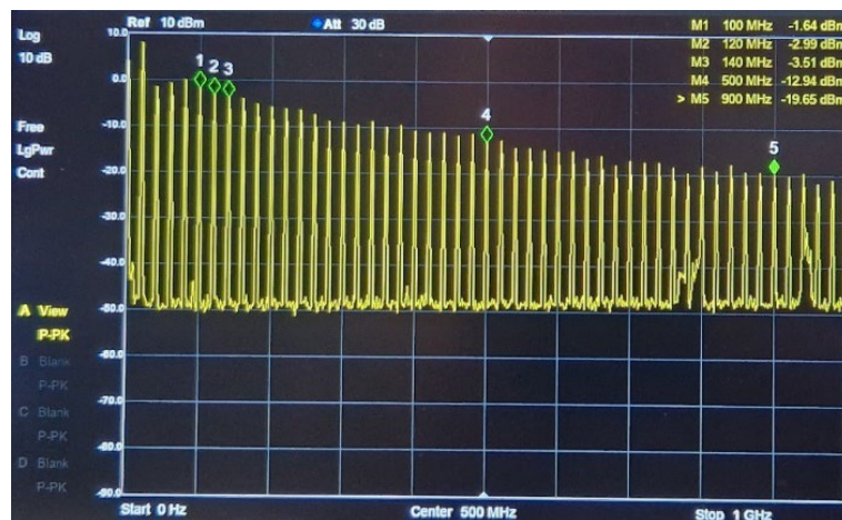
Figure 17: Spectrum of the signal source (comb generator and amplifier).
