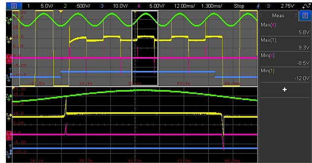
Figure 43: Circuit waveforms for TRIAC driven by ZC opto-triac zoomed in on TRIAC conduction cycles with resistive load ( V_{TR} (I), V_{TR} (I), I_{OT} (I), V_{Rled} (I)) (DANGER: HIGH VOLTAGE)
