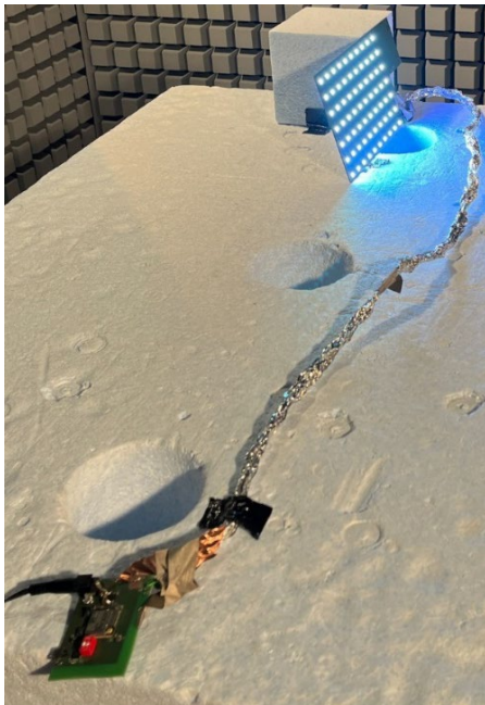
Figure 21: Cable between MCU-PCB and LED-Panel shielded with aluminium foil.
