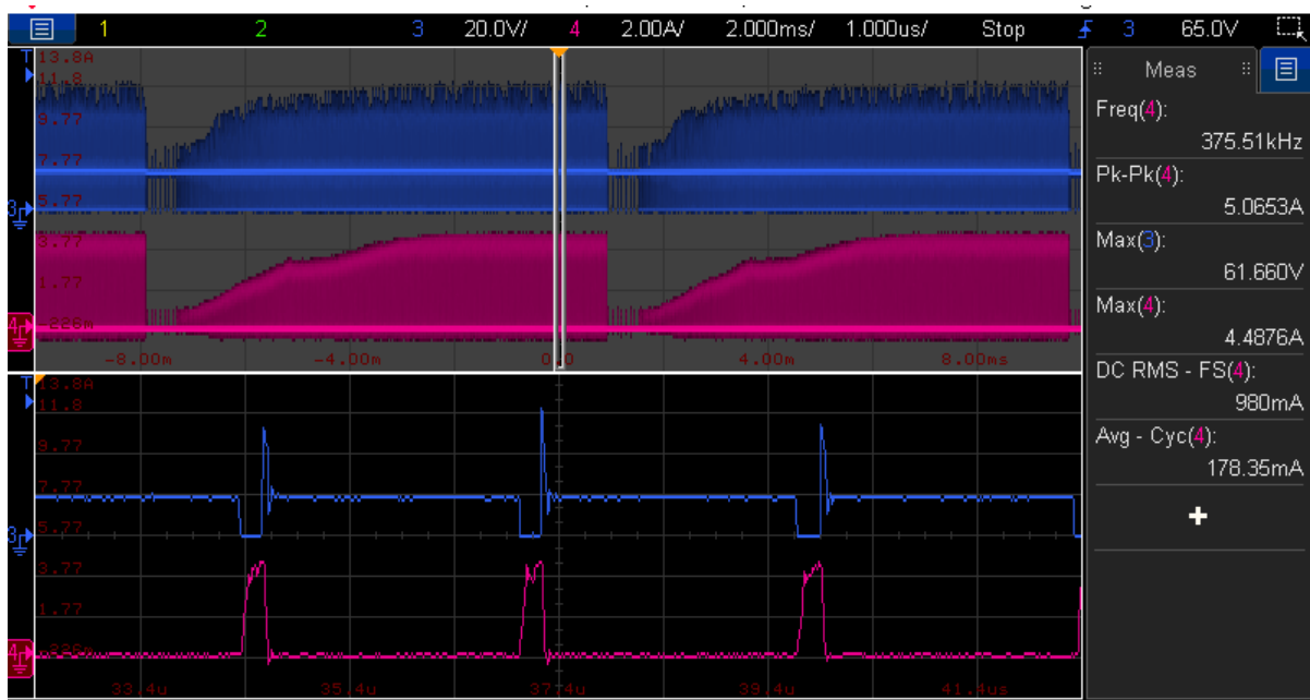
Figure 29: Short-circuit protection at V_{in} = 18 V
