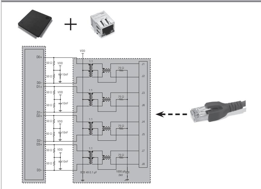
Fig. 4: Power over Ethernet Base-T
