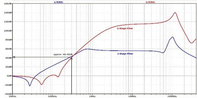
Figure 17: LTspice simulation of CM insertion loss, 10 kHz to 400 MHz; blue = single-stage filter; red = Two-stage filter.
