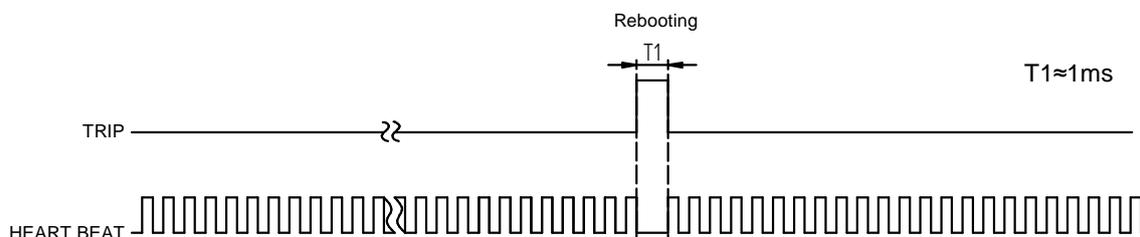
Figure 15: Watchdog function diagram for 791002002
