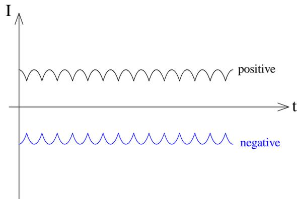
Figure 8: three phase pulsating DC characteristics
