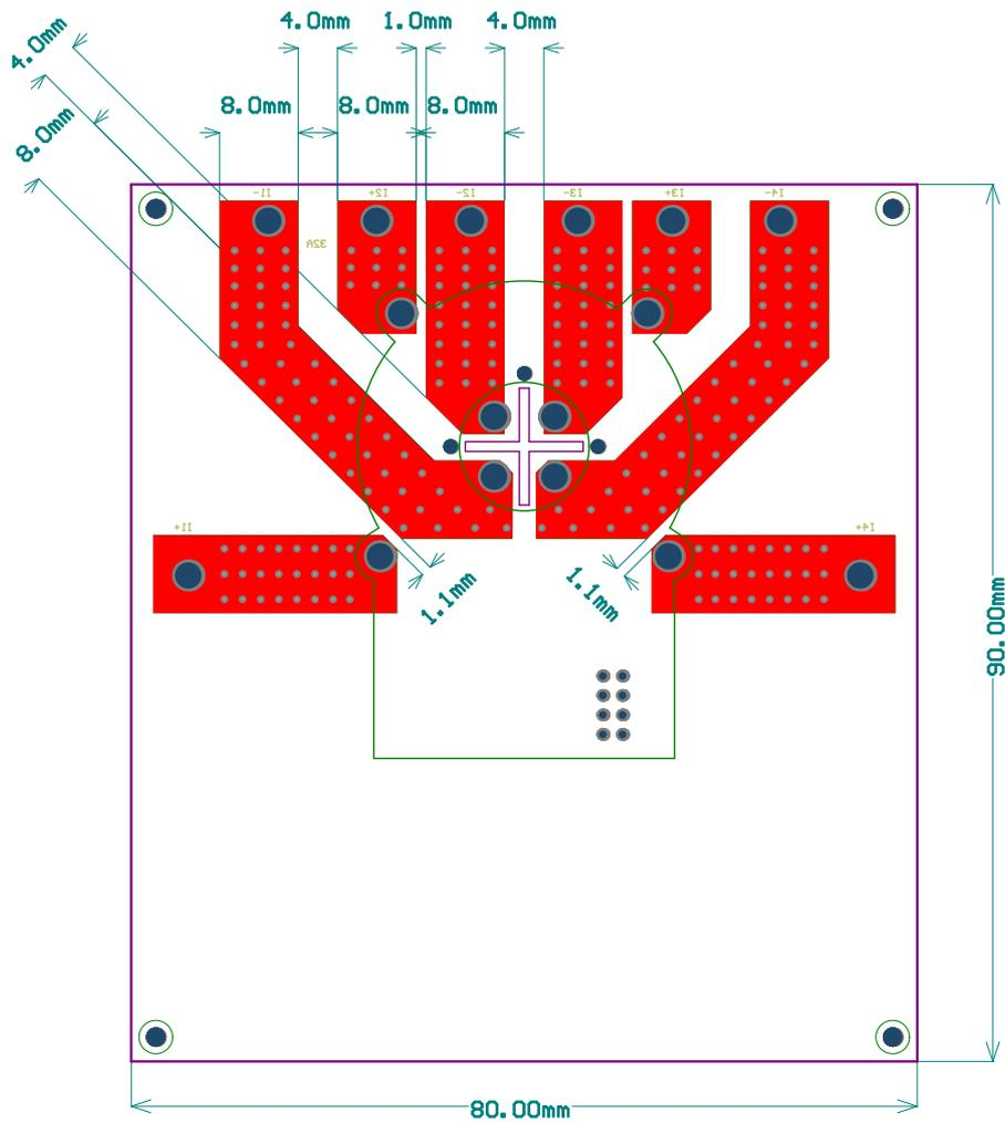
Figure 20: PCB Trace Layout design example 1
