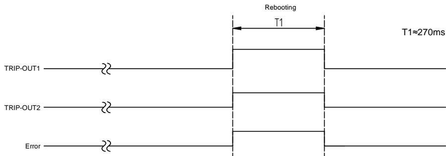
Figure 16: Watchdog function diagram for 791002004
