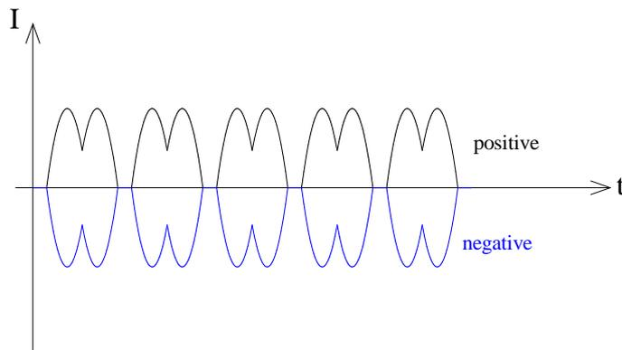
Figure 7: two phase pulsating DC characteristics
