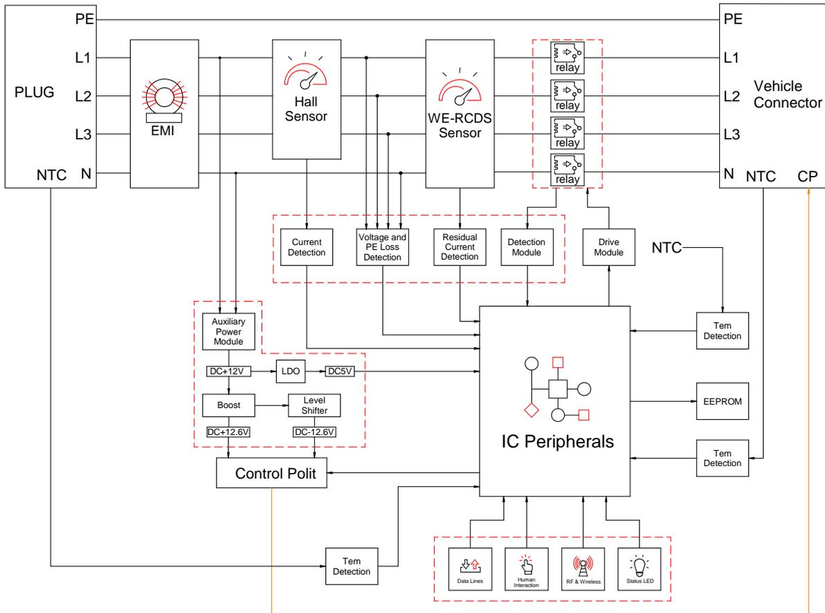
Figure 2: Simplified typical block diagram of Mode 3 EV charging station
