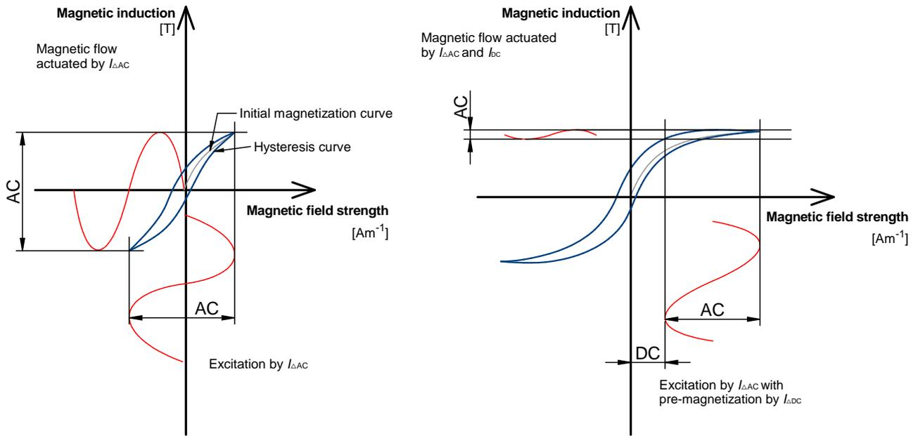
Figure 4: Magnetization by AC and DC
