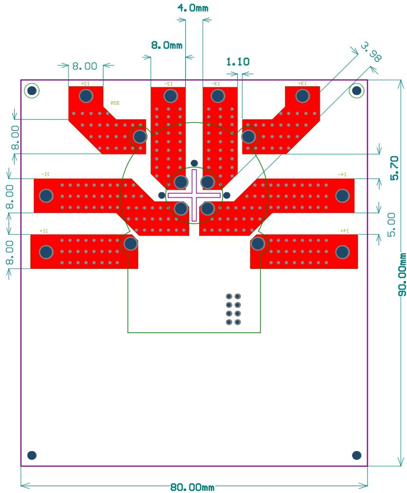
Figure 21: PCB Trace Layout design example 2 with improved temperature characteristic
