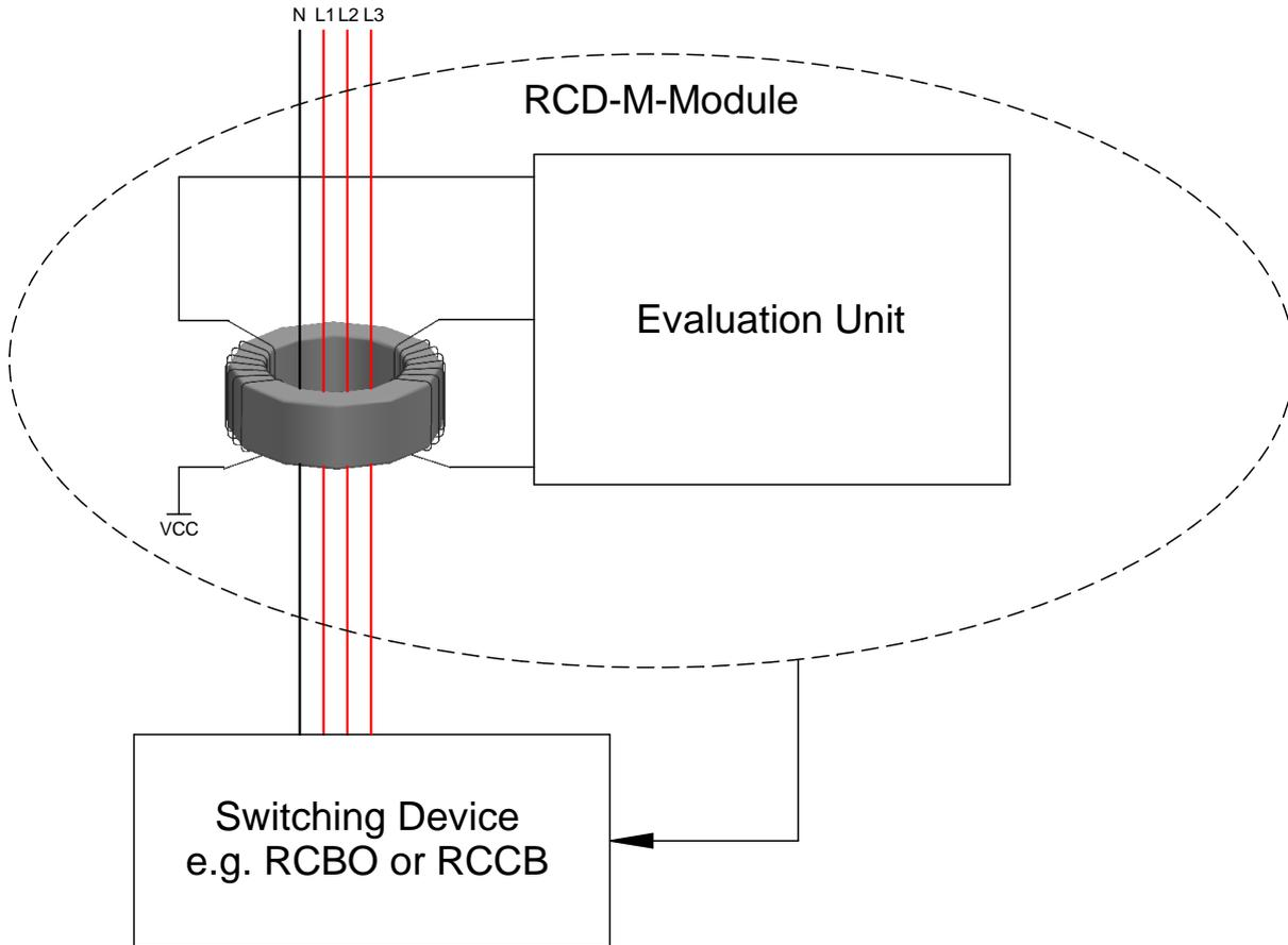
Figure 5: RDC-M-module schematic
