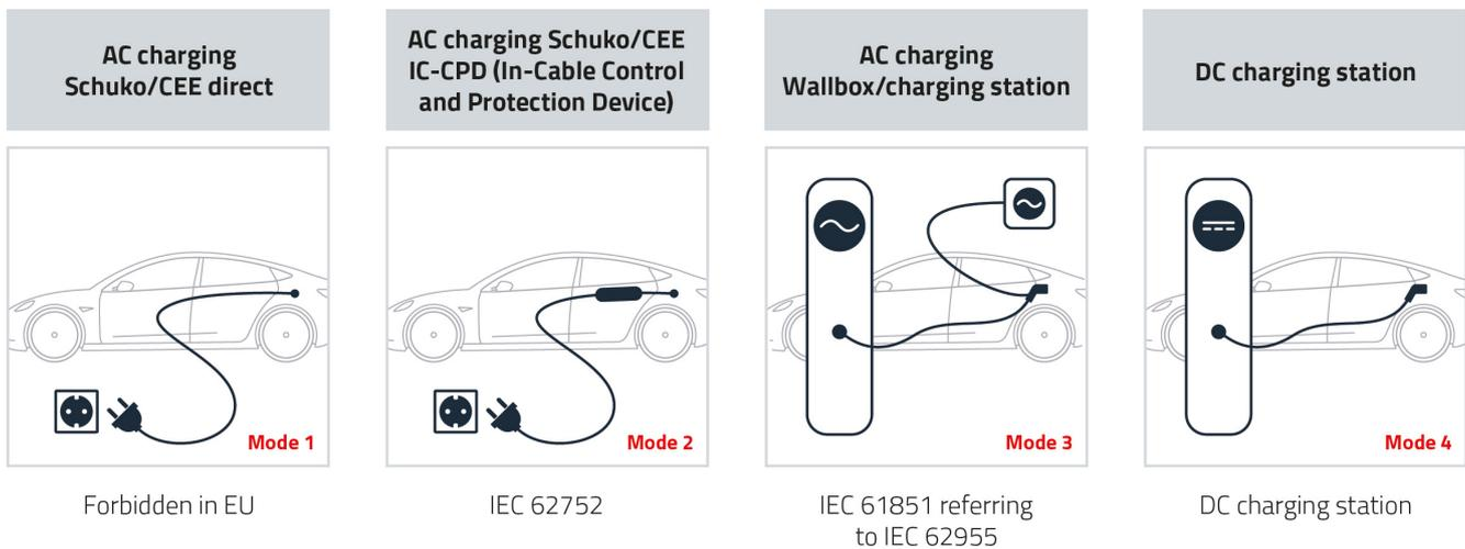
Figure 3: Different charging modes as defined in IEC 61851-1
