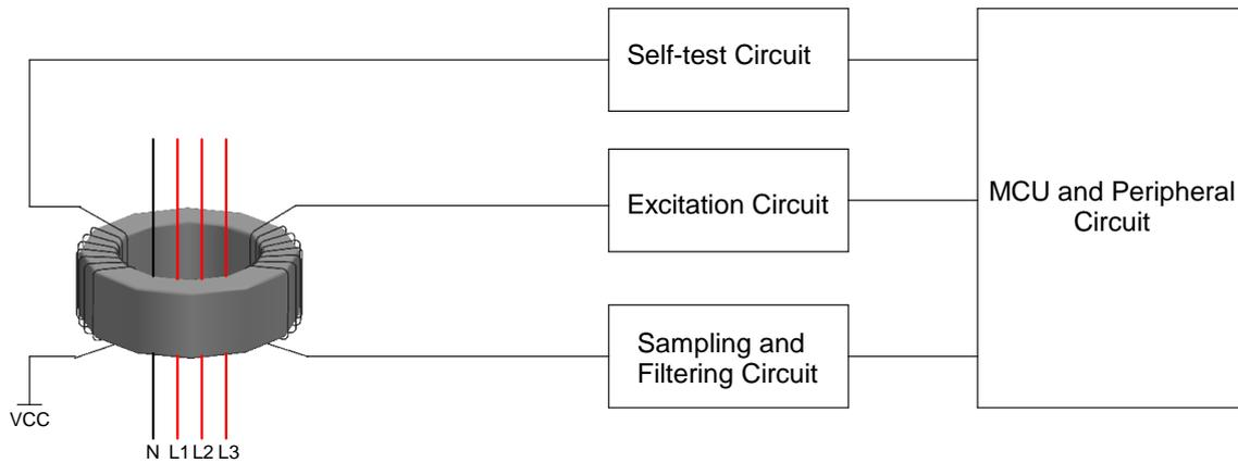
Figure 1: Block diagram
