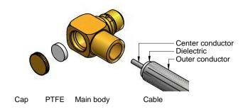
Step 2. Insert cable into connector main body until cable dielectric is attached to connector internal positioning point Check and make sure cable center conductor sits inside solder slot Solder cable center conductor using minimum amount of solder paste (check point 2)
