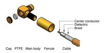
Step 2. Please slide ferrule onto cable and splay out cable braid
