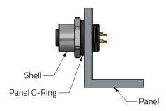
**Step 3.** Tigthen Panel Nut. Recommended tightening torque: 10-15 kgf-cm
