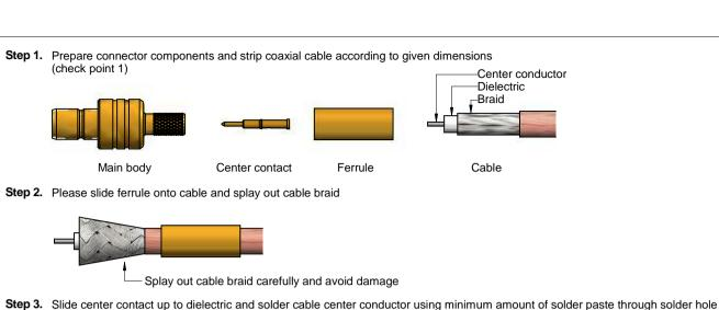
(check point 2) The gap between center contact and dielectric has to be as small as possible
