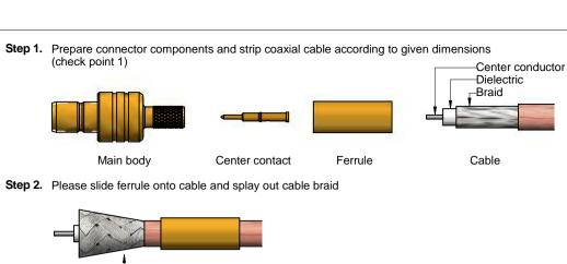
Splay out cable braid carefully and avoid damage
