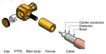
Step 2. Please slide ferrule onto cable and splay out cable braid
